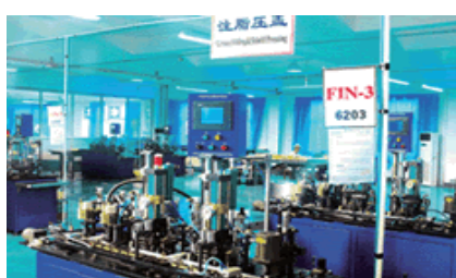
Gease filling & shield pressing line
