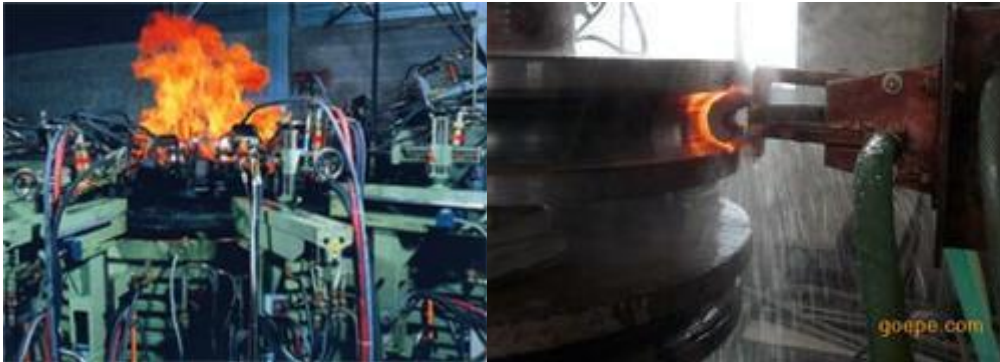
Sketch of raceway nest quenching
